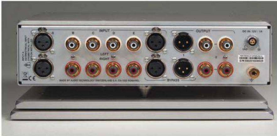
One pair balanced and four pairs single-ended inputs; one pair balanced and two pairs single-ended outputs.
